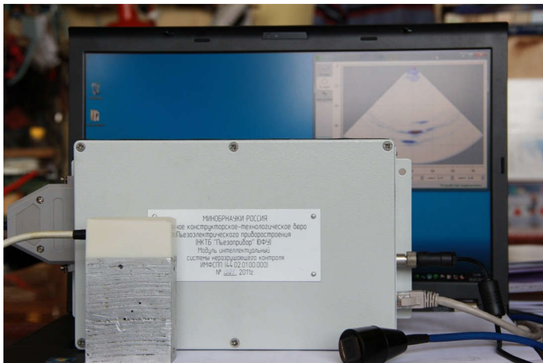
A prototype of an intelligent distributed nondestructive testing system SNTS with an ultrasonic antenna array installed on the control object, and a computer that performs the function of a monitoring post that displays the results of the control
